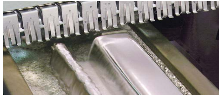
Turbulent wave for SMD and laminar wave for through-hole soldering.
