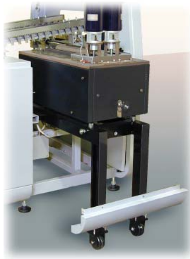
Motorized roll-out pot provides easy access.
