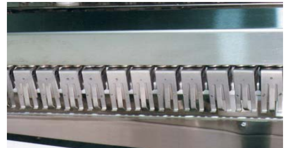
Finger conveyor with "L" finger for pallet or pallet-less operation.
