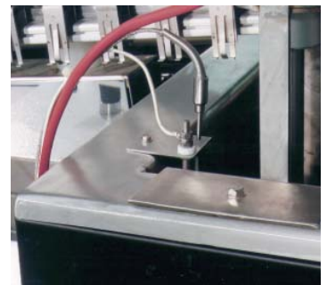
Solder level sensor with alarm
